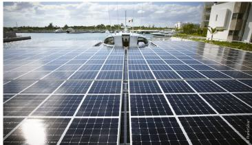
kinetic energy transmitted through the hull of the vessel. Sikaflex®-292 has been proving its reliability on a major voyage, protecting the rigid photovoltaic modules against fractures on the flexible hull of the "Tûranor PlanetSolar".
