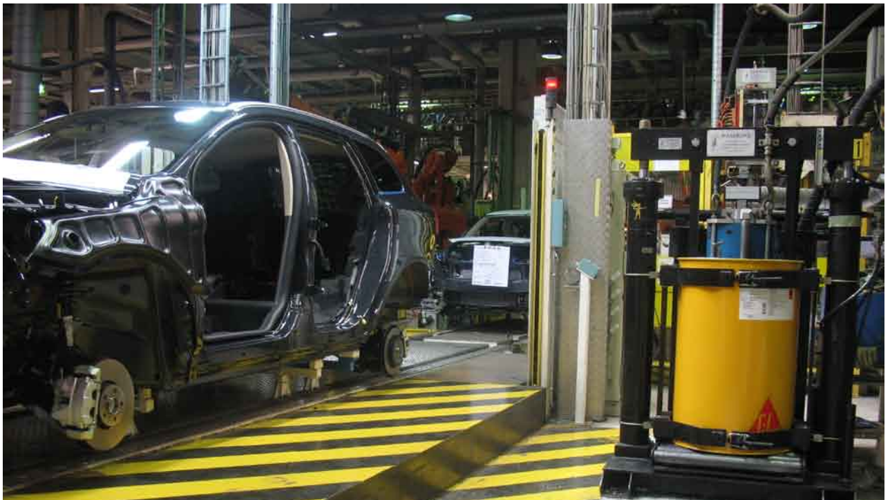
The PUR direct glazing cell located at Volvo Car Corporation's Gent facility in Belgium. Photo from February 2010.
