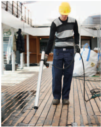
Fig. 18 Applying Sikaflex®-290i DC
