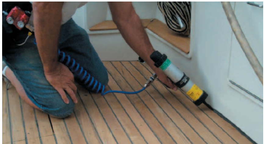
Fig. 27 Sealing the edges after renovation with Sikaflex®-295 UV
