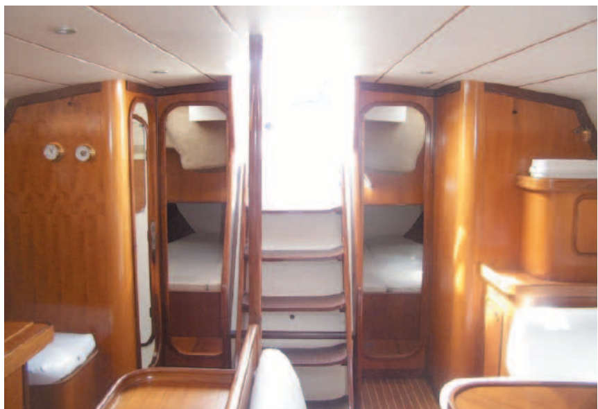
Fig. 4 High-quality lightweight panels finished in traditional high-gloss wood veneer and bonded using Sikaflex®-292i
