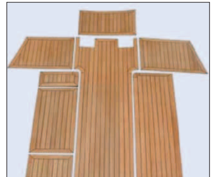
Fig. 23 A prefabricated teak deck is laid out in preparation for fitting
