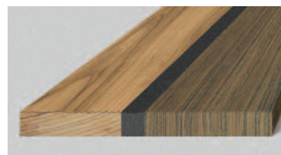
Fig. 1 Left side: laying year rings are not recommended. Right side: standing year rings are best.
