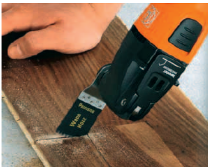
Fig. 48 Cutting planks with vibrating knife
