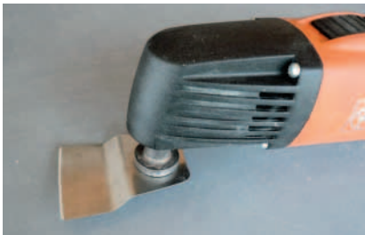
Fig. 47 A useful and effective vibrating scraper power tool
