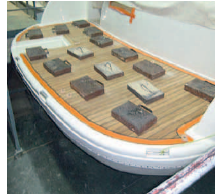
Fig. 26 Holding in place with weights
