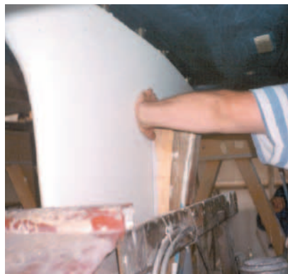
Fig. 1 A keel is carefully slid into position
