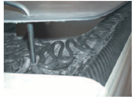
Fig. 2 A locating pin ensures perfect alignment
